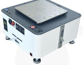
K-AM Moment of Inertia Measurement Systems are products with advanced features and user interface which can measure the inertia moments of objects of various weights and sizes in a single axis.
